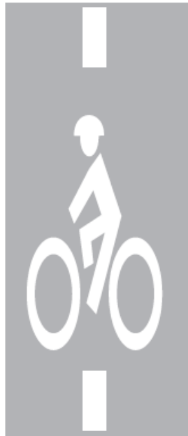
Figure 1-34: Bike symbol for loop detection placement
